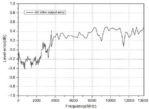
Measured at -60 dBm, level error vs frequency
