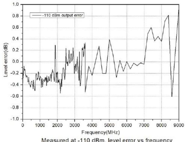
Measured at -110 dBm, level error vs frequency
