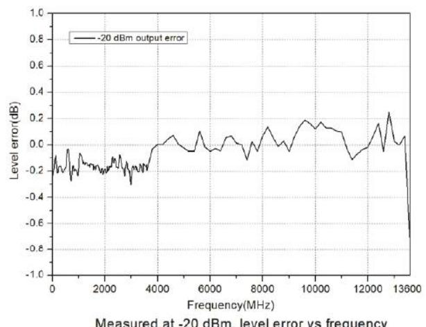
Measured at -20 dBm, level error vs frequency
